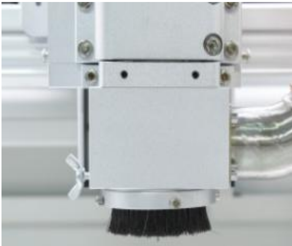
Adopt the top dust collection design, equipped with anti-static brush adsorption, ensure the PCBA surface clean
